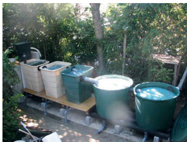
Above: Filtration systems using biomedia, made from garden waste bins © D.R.
