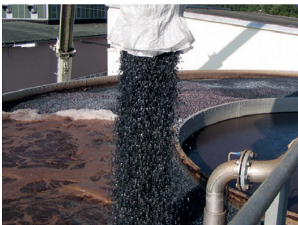
Above: Adding biomedia to a reactor © D.R.
